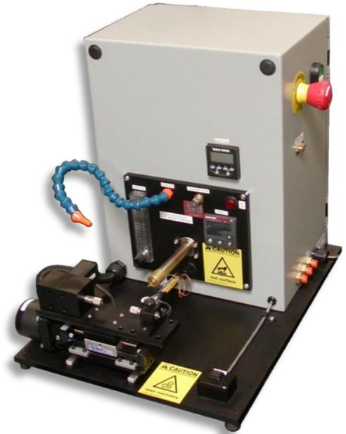
Bonding inconsistencies due to operator variability become a non-issue with AVID Innovation's AHB200 series AutoBonder. This automated hot box not only delivers a precisely controlled stream of hot air to bond or shape your catheter parts, but it holds, rotates and translates the catheter under the hot air stream in precisely the same way... every time.
